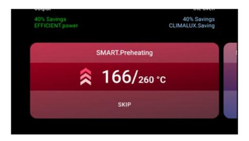
UNOX recommends that you use SMART. Preheating, an automatic preheating program that autonomously sets the preheating time and temperature; it also takes into account the dispersion of heat when you open the door and is activated when the oven moves from one step to the next, adjusting the oven cavity to the step's new parameters.
