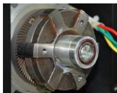
Step 7 –remove the bearing cover
