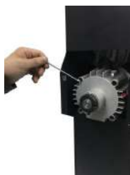
Step 5 – release grinding house
