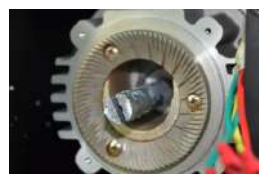
Step 9 – remove the disk holder
