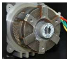
Step 8 -remove the shear key
