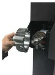
Step 6 -remove grinding house
