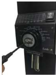
Fig 8-2 loosen the securing screws
