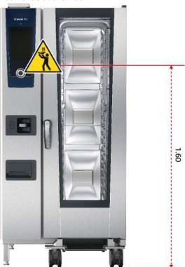
If your cooking system is installed such that the top rack level is more than 1.60m off the floor, the warning sign included in delivery must be affixed here.
